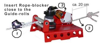
and **Rolls A and B**, close the **Safety-clamp**. Take away the **Rope-blocker** from the power-strand. Continue roping down while carefully guiding the knot around the **Brake-block**. Stop roping down just before the knot reaches the guide-rolls, open the upper guide, let the knot pass and close the guide-roll again. (probably you will need to push the rope downwards against the lower guide-roll). Continue roping down as usual
