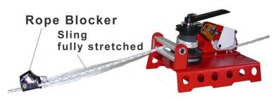
Take the **Rope-blocker** out of its box and pull out until the **Sling** is fully stretched, then hang it into the power-strand and **close** it. Pull slightly back at the retarding-strand and fully open the **Safety-clamp** by
