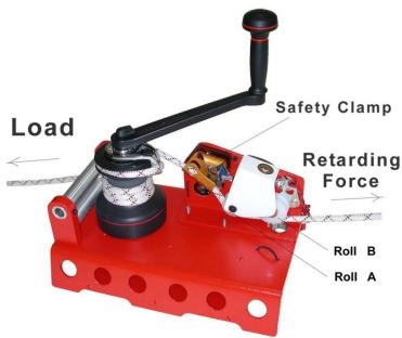
To start roping down apply load at the power-strand of the rope, then pull back slightly upwards at the retarding strand of the rope and hold the rope back. This movement opens the **Safety-clamp** -> the roping down can start.
