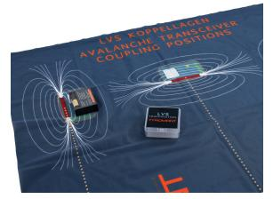
The **avalanche transceiver training tool** is used for the theoretical handling and understanding of the work and effect of an avalanche transceiver.
